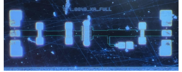
Fig. 6. Detail of the UMS GH-15 pre-matched transistor
